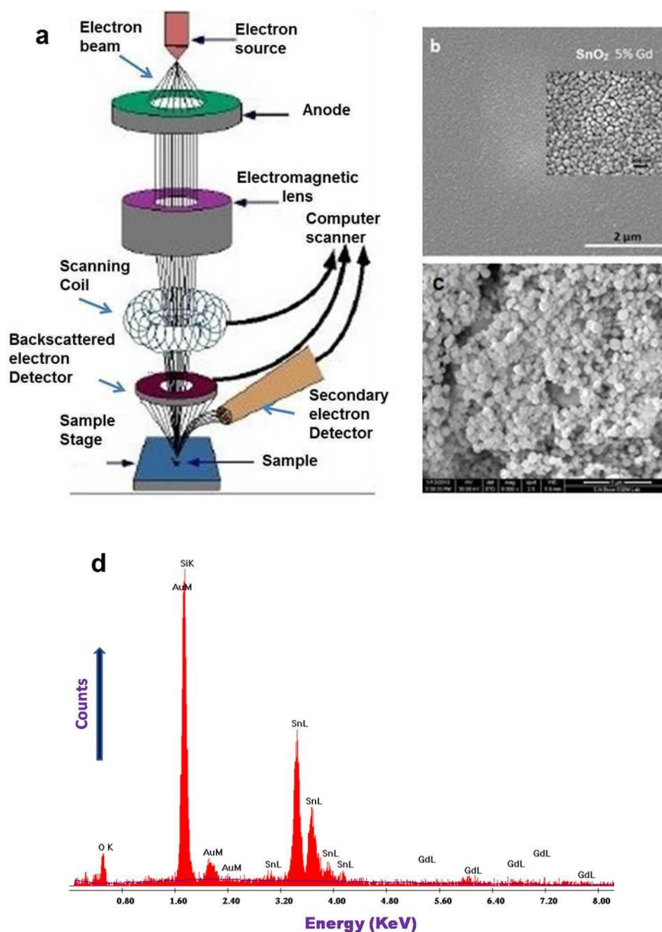
Fig. 2.16: (a) Schematic diagram of SEM components; SEM image of (b) Gd-doped \text{SnO}_2 thin film and (c) Co-doped \text{SnO}_2 .
